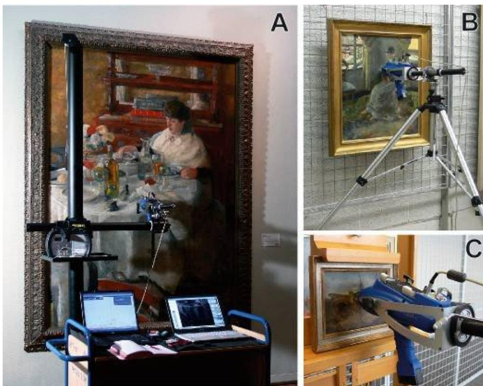
*Fig. 1: (A) The PXRf instrument mounted on a studio camera stand during analysis of 'The lady eating oysters' (1882) in the Museum of Fine Arts, Antwerp, Belgium; (B) The PXRf installed on a lighter tripod during analysis in the depot of the Royal Museums of Fine Arts Brussels; (C) the relatively large analysis spot of ca. 1 cm<sup>2</sup> can render the analysis of small sized paintings and/or finely painted compositions with small colour areas difficult.*
